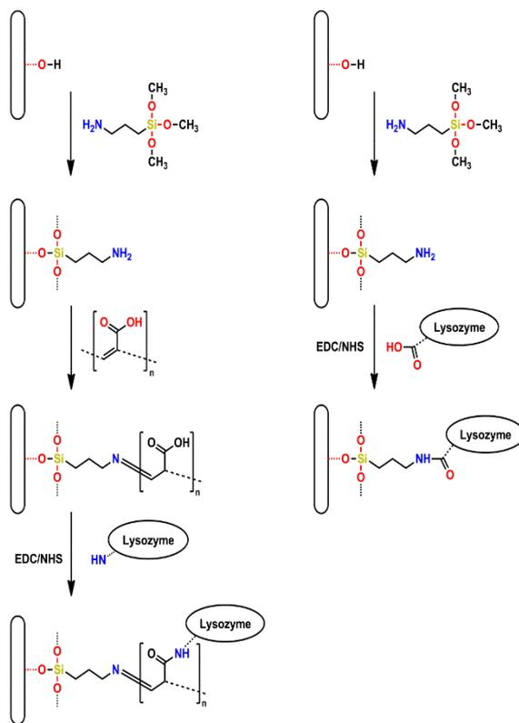
**Figure 1.** Reaction scheme for the immobilization of lysozyme on steel surface. The amine groups in the sol-gel network are utilized for the addition of carboxyl groups and then the covalent binding of lysozyme from its amine-end (left) or for the direct
