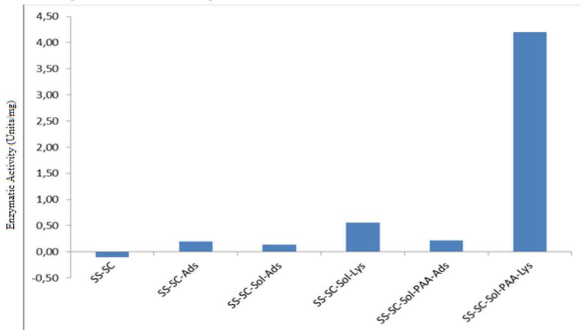
**Figure 2.** Enzymatic activity of six different stainless steel coupons. (Ads refers to the adsorbed lysozyme on the coupons)
